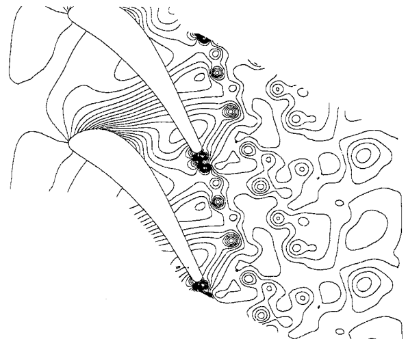
Fig. 9 Instantaneous pressure contours for laminar flow.
